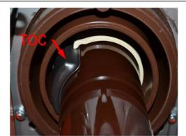
Fig. 2 Adapted TOC sensor with clamp ready for operation
